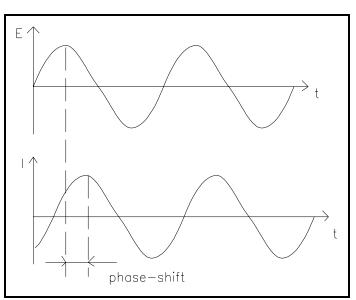
Figure 2-1 Sinusoidal Current Response in a Linear System
