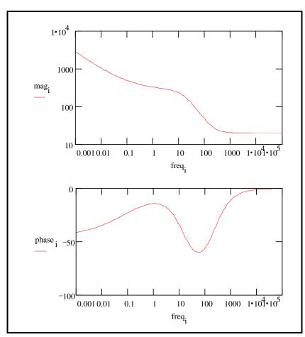
2-20 Bode Plot for the Mixed Control Circuit
