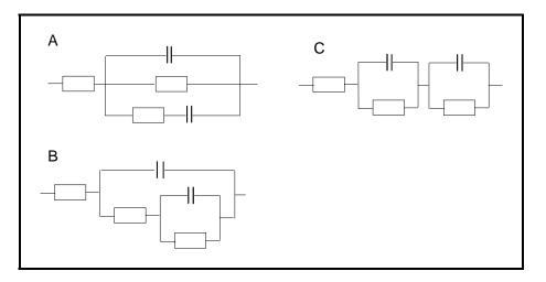
As you can see, there is not a unique equivalent circuit that describes spectrum. You therefore can not assume that an equivalent circuit that produces a good fit to a data set represents an accurate physical model of the cell.
