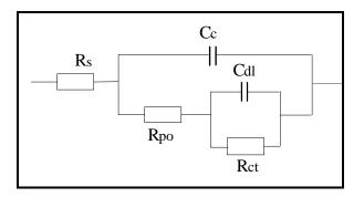
When you use EIS to test a coating, you fit a data curve to this type of model. The fit returns estimates for the model parameters, such as the pore resistance or the double layer capacitance. You then use these parameters to evaluate the degree to which the coating has failed.
