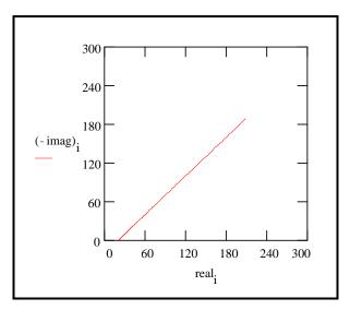
The same data is plotted in the Bode format in Figure 2-17. The phase angle of a Warburg impedance is  $45^{\circ}$ .
