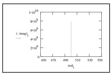
The value of the capacitance cannot be determined from the Nyquist plot. It can be determined by a curve fit or from an examination of the data points. Notice that the intercept of the curve with the real axis gives an estimate of the solution resistance.
