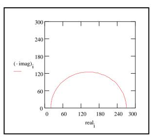
Figure 2-14 Nyquist Plot for 1 mm/year Corrosion Rate
