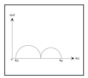
This spectrum can be modeled by any of the equivalent circuits shown in Figure 2-25.
