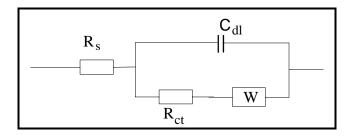
This circuit models a cell where polarization is due to a combination of kinetic and diffusion processes. The Nyquist plot for this circuit is shown in Figure 2-19. As in the above example, the Warbug coefficient is assumed to be to be about 150. Other assumptions:  $R_s = 20 \Omega$ ,  $R_{ct} = 250 \Omega$ , and  $C_{dl} = 40 \mu$ F.
