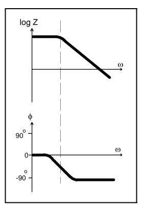
Figure 2-5 Bode Plot with One Time Constant
