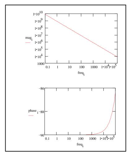
Figure 2-13 Typical Bode Plot for an Excellent Coating
