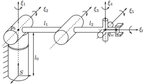
Figure 5: Elbow manipulator.
