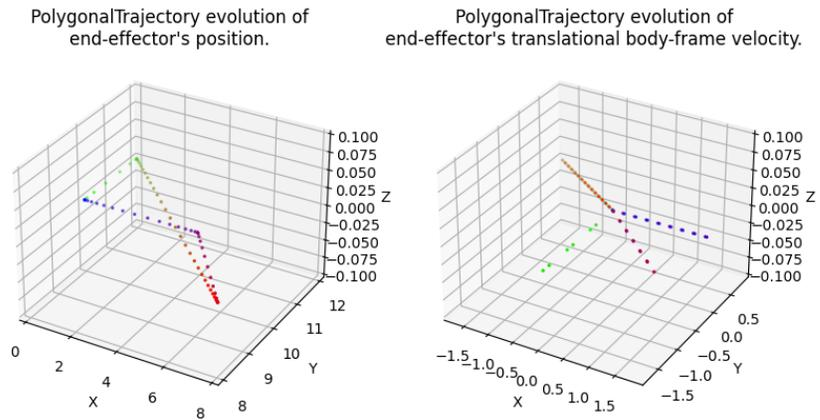
Figure 4: Example polygonal trajectory with 4 goal points.
