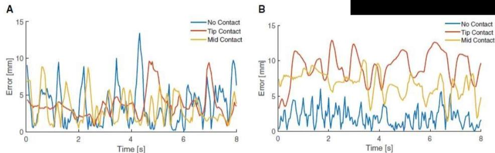
Fig. 4. Error plots for tracking. (A) With the soft cPDMS sensor. (B) With the commercial flex sensor.
