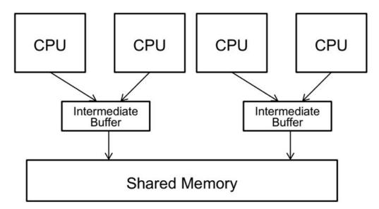
A system where a write by one processor becomes visible to a subset of other processors before it becomes visible to all processors
