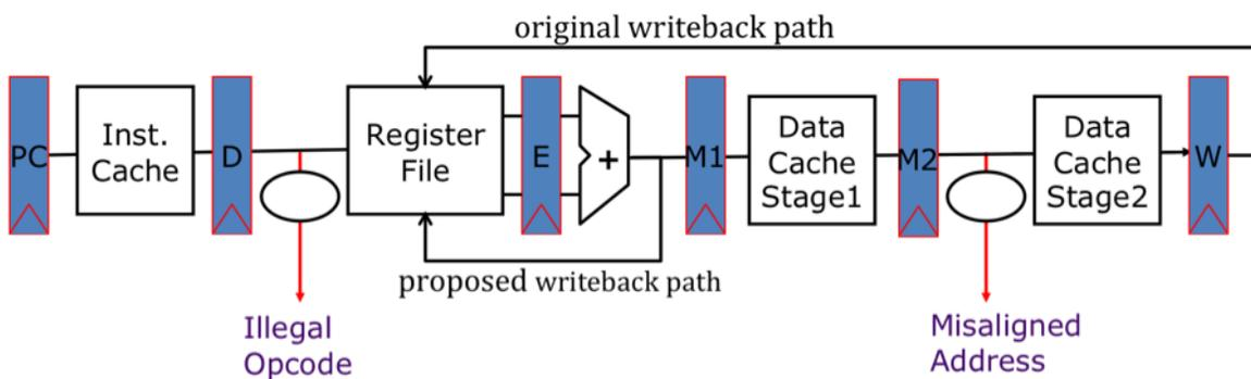
Figure 1-B. 6-stage pipeline with proposed additional write port.
