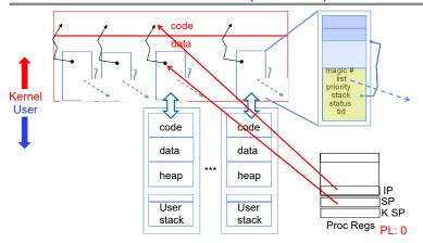
switch\_threads: save regs on current small stack, change SP, return from destination threads call to switch\_threads
