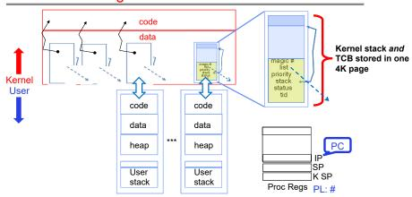
• Each user process/thread associated with a kernel thread, described by a 4KB page object containing TCB and kernel stack for the kernel thread
