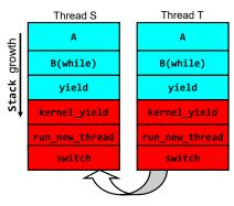
Thread T's switch returns to Thread S
