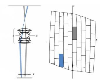
2. A slice of the sampled light field at a single location on the *u* plane in the plenoptic camera diagram is typically called a sub-aperture image. Describe in your own words what this slice of the light field represents and how it should appear.
