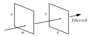
1. In the diagram of a plenoptic camera below, which two planes define the light field parameterization? Which components of the camera determine the sampling resolution for each of these planes?
