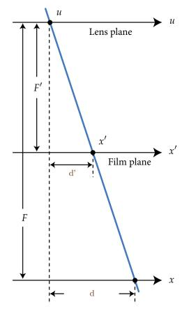
2. Combine this derivation of the reparameterized camera light field with the imaging equation that expresses the recorded image as the irradiance on the sensor plane to derive the computational refocusing equation that expresses how the recorded light field can be reparameterized and integrated to compute images refocused to different depths.
