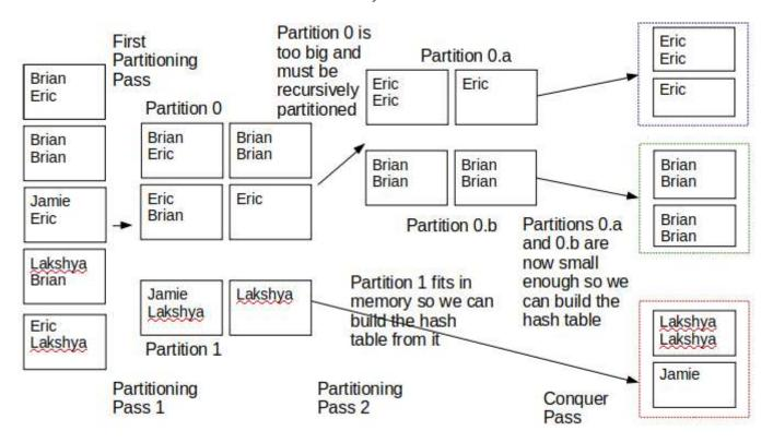
After the first partitioning pass (Partitioning Pass 1), Partition 0 is 4 pages, and Partition 1 is 2 pages. Partition 1 fits in memory, but Partition 0 does not. This means we must recursively partition Partition
