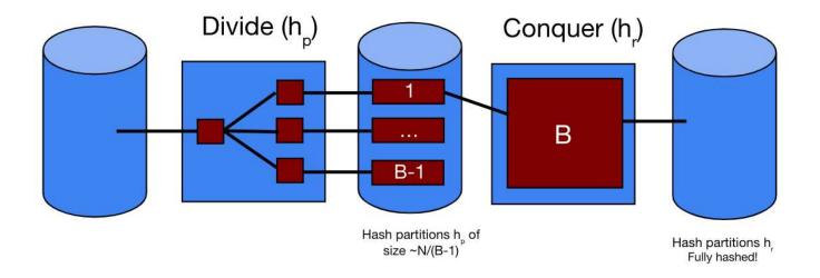
The image below shows recursive partitioning. Notice that the additional phases only apply to the partition with size greater than B pages (grey partition).
