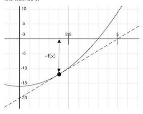
A newton\_update expresses the computational process of following this tangent line to 0, for a function f and its derivative df.
