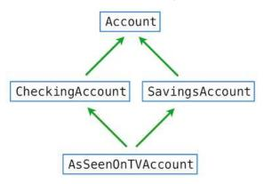
For a simple "diamond" shape like this, Python resolves names from left to right, then upwards. In this example, Python checks for an attribute name in the following classes, in order, until an attribute with that name is found:
