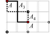
Net Constraints:  $x_{A1} + x_{A2} + x_{A3} + x_{A4} \le 1$ Variable Constraints:  $0 \le x_{A1} \le 1, 0 \le x_{A2} \le 1$ ,  $0 \le x_{A3} \le 1, 0 \le x_{A4} \le 1$
