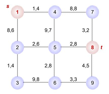
Find the shortest path from source **s** to target **t** where the path cost  $\sum w_1 + \sum w_2$  is minimal
