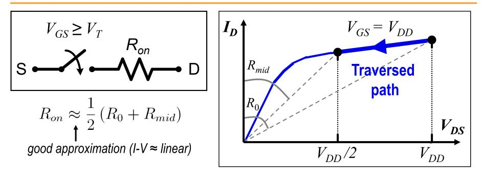
$$R_{on} = \frac{1}{2} \left( \frac{V_{DD}}{I_{DSAT} \cdot (1 + \lambda V_{DD})} + \frac{V_{DD}/2}{I_{DSAT} \cdot (1 + \lambda V_{DD}/2)} \right)$$
