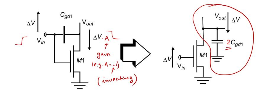
"A capacitor experiencing identical but opposite voltage swing at both terminals can be replaced by a capacitor to ground, whose value is two times the original value"
