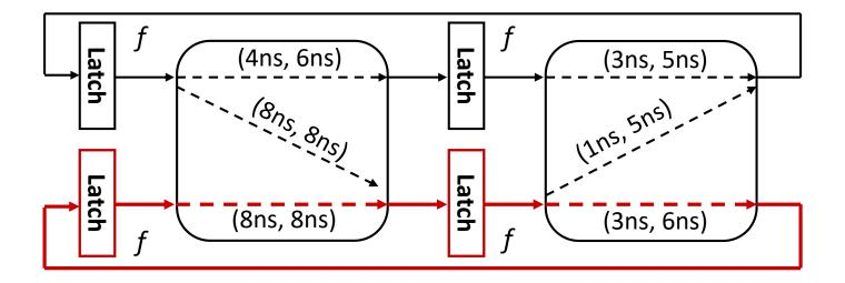
$T_{cycle} \ge 8n + 6n + 2*0.5n = 15n \text{ (over 2 cycles)}$   $T_{cycle} \ge 7.5ns$
