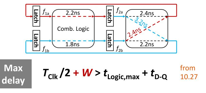
Latch  $f_{1b}$  must latch in the data from  $f_{2a}$ • W > 3.2ns + 0.2ns – 2.6ns = 0.8ns
