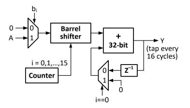
Throughput =  $(t_{add} + t_{mux} + t_{shift})/16$
