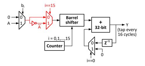
If MSB  $b_{15} = 1$ , then invert A and add. The inputs A and B do not change for 16 cycles.
