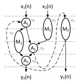
Schedule requires two multipliers and one adder. Two pipeline stages in the multipliers can be used independently in the same cycle ( $M_1$  in cycle 2).
