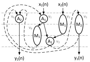
Solution will depend on the retimed version in part (c). For the retimed version shown in (c), the scheduled graph is shown here. We need two multipliers and two adders.
