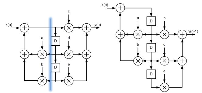
Prove the two circuits have equivalent functionality (circuit on the right has one-cycle latency). (4 pts)
