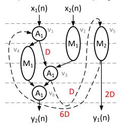
c) Pipeline the original flow graph by inserting one register at both inputs. Now retime the pipelined graph so as to ensure minimum delay.
