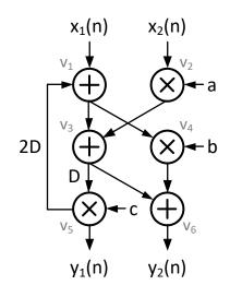
a) Schedule this graph using a maximum of 2 adders and 2 multipliers as available resource units. Assume that the multipliers are 2-stage pipelined and the adders are single stage pipelined in your scheduling. Clearly draw the scheduled graph indicating the time steps and the hardware allocation for the operations  $v_1 - v_6$ . How many cycles (N) do you need to complete the schedule? Use as many rows in the table below as necessary.
