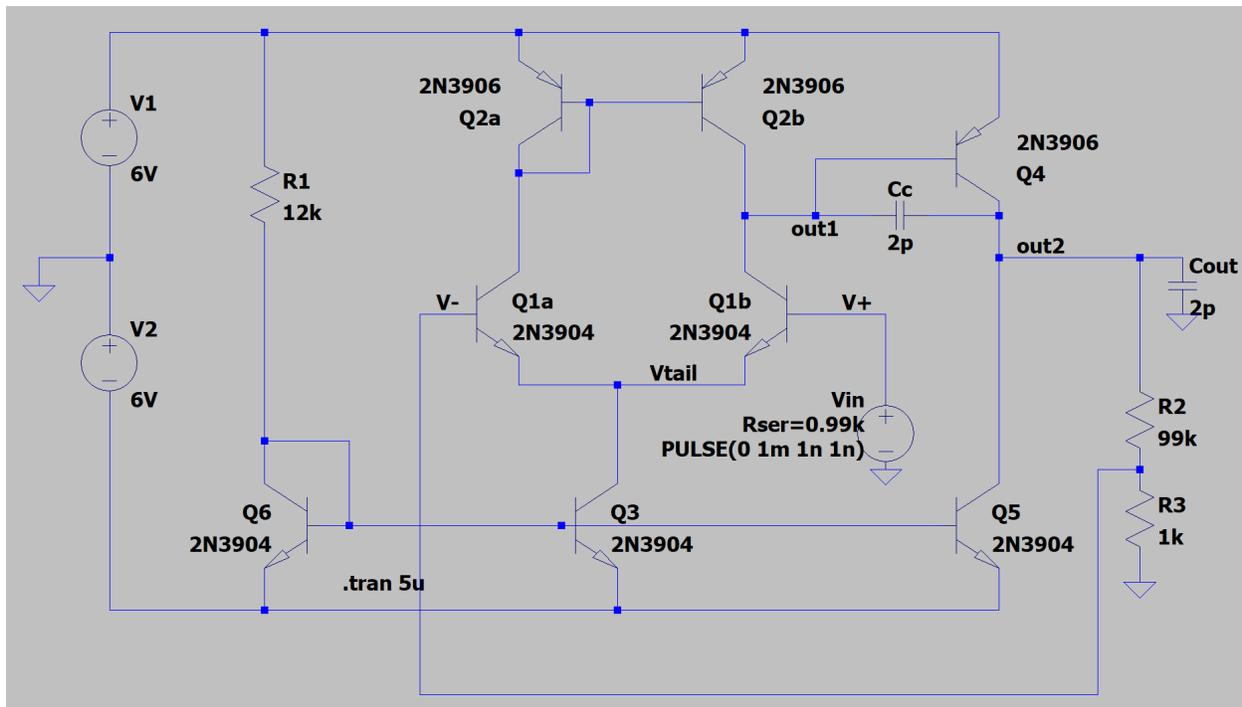
Figure 2: The op-amp in resistive feedback. Capacitors  $C_C$  and  $C_{out}$  represent typical parasitics for a breadboard. (Note that I changed  $V_{in}$  to have a source resistance of  $0.99\text{k}\Omega$  to match the feedback network, to avoid the effect of input bias current. This does not necessarily hold for CMOS.) [File: BJTtopamp101xFB.asc]
